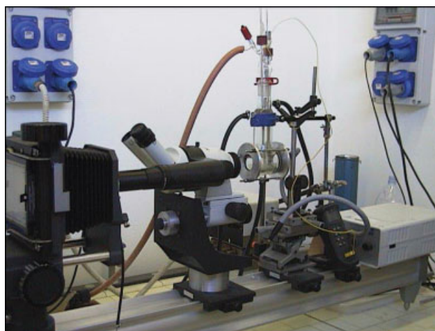
Figure 1 Experimental apparatus used: from the left, the camera, the microscope and the jacketed glass chamber can be seen. [Color figure can be viewed in the online issue, which is available at www.interscience.wiley.com .]
